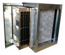
power supply is housed in a hinged power door and is sealed from the airstream. The ESP includes a 1" thick pre and post aluminum mesh filters. The ESP can either supplied in manual wash type or auto wash type as per the project requirement. A drain pan and drain connection can be provided in the cabinet if required for removal of excess oil and grease flowing down if the cells are not cleaned in time.
