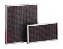
the exhaust air. The metallic filter is washable type and requires regular maintenance by washing the filter in a solution of detergent & warm water and dried with compressed air. The average life of these filters (if maintained correctly) is 2 to 3 years.
